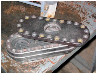
Training contents with practical relevance and value: a spinning Jet from the Nylon plant...
